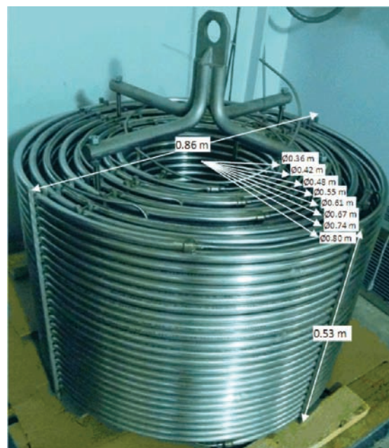
Figure 2. Pilot-scale 73 L coiled-tube reactor.
